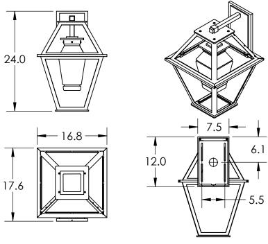
Mounting Method: Mounts To Building Structure
